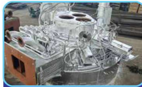
Roof of LF Furnace
